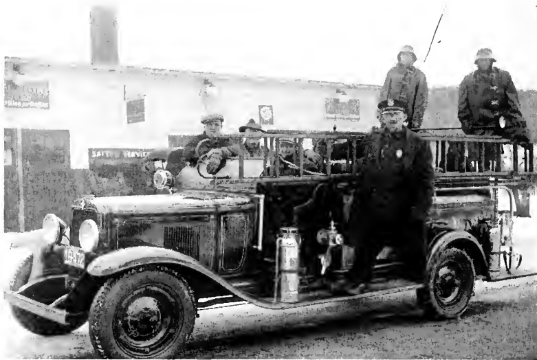
82-M1 1929 Chevy 1 1/2 Ton, 6 Cylinder Fire Truck built by Wachusett Motors.
